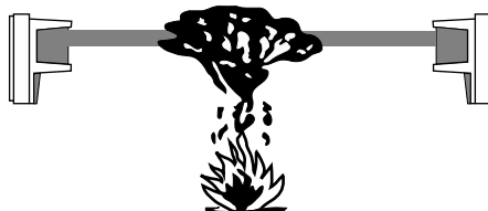
Figure B - Beam obscuration
